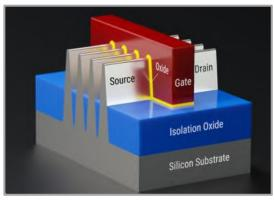
Chips utilizing FinFET have been on the market since the first half of the 2010s with Intel commercializing 22nm FinFET in 2011. With continuous optimization of the transistor density per chip, it has become the dominant design at 14nm, 10nm, 7nm and 5nm process nodes. The state of the art in FinFET is nominally 5 nm today, produced by TSMC and Samsung, with 3 nm in pre-production. Although European companies design in FinFET, they rely on foundries such as TSMC and Samsung for
