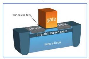
of optimizing power consumption when speed is less critical. Due to its planar structure, FD- SOI manufacturing is less complex requiring fewer process steps than FinFET.
