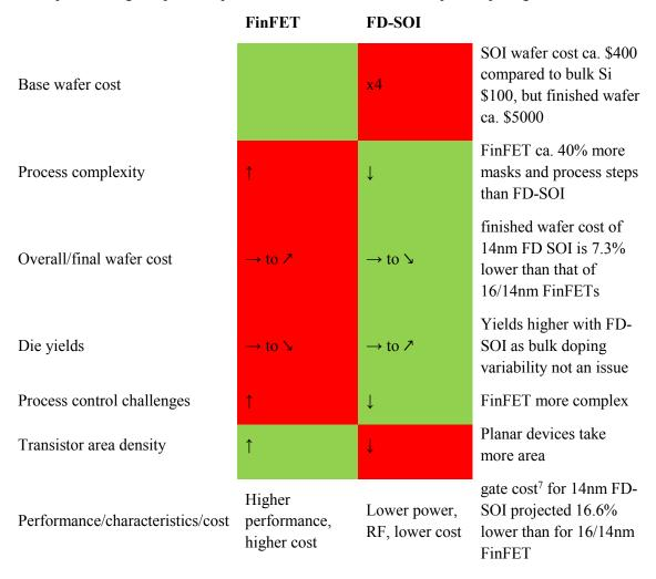
However, FD- SOI is well suited to achieving a **better performance** / **power consumption trade-off at functionally equivalent nodes.**<sup>8</sup> It is fair to say that the two technologies compete in many applications including automotive, AI, IoT, 5G/6G, and industrial manufacturing.
