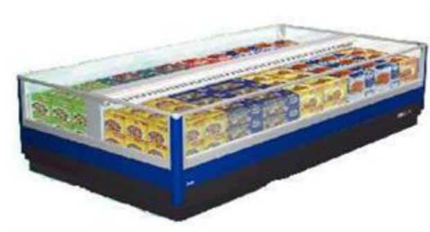
Figure 8 Open remote horizontal island for frozen products (category RHF4 according to EN ISO 23953), with 2.9 m 2 TDA, operating in temperature class L1 (-18°C to -15°C), using R404a as refrigerant, with a product life of 9 years. Energy consumption: 32.2 kWh/day
