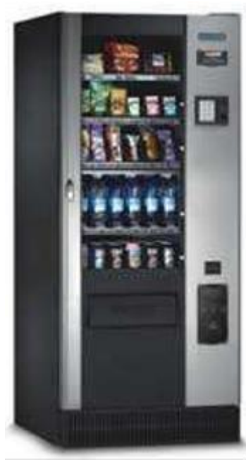
Figure 11 Spiral vending machine, with a net volume of 750 litres, operating in temperature class M2 (-1°C to 7°C), using R134a as refrigerant, with a product life of 8.5 years. Plug-in. Energy consumption: 7.1 kWh/day
