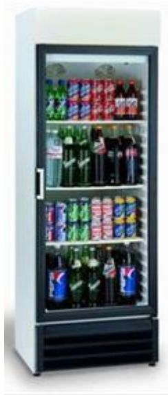
Figure 9 Beverage cooler with one glass door, operating at temperature classes H1 (1°C to 10°C), with a net volume of 500 litres, using R134a as refrigerant, with a product life of 8 years. Plug-in. Energy consumption: 7.5 kWh/day
