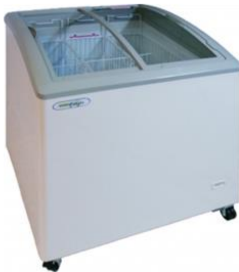
Figure 10 Packaged horizontal ice cream freezer with lids (category IHF6 according to EN ISO 23953), with a net volume of 291 litres, operating in temperature class L1 (-18°C to -15°C), using R507 as refrigerant 53 , with a product life of 8 years. Plug-in. Energy consumption: 3.6 kWh/day
