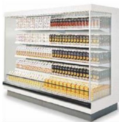
Figure 7 Open vertical multi-deck remote refrigerating display cabinet for chilled products (category RVC2 according to EN ISO 23953), with 5.25 m 2 TDA, operating in temperature class M2 (-1°C to 7°C), using R404a as refrigerant, with a product life of 9 years. Energy consumption: 56.9 kWh/day
