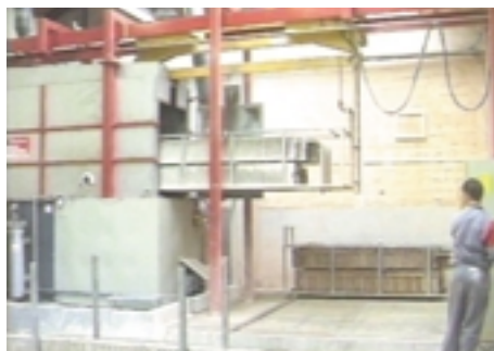
Example of a closed blasting cabin co-financed by a CRAM. Use of water-based cleaning product with a closed circuit recycling system.
