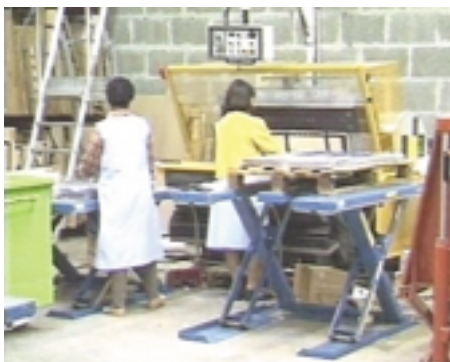
Example of a working station laying-out co-financed by a CRAM. It is about cardboard cutting with a protective device consisting in a mobile wire fenced casing associated to a sensitive bar and a lifting table for the handling of cardboard at a constant height.
