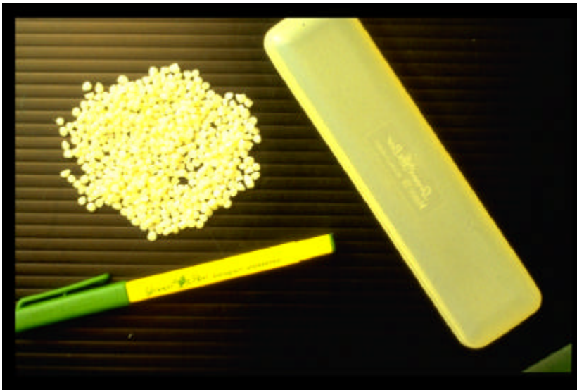
Figure 4: A pen and case made from maize-based biopolymer. The injection moulding granules are top left
