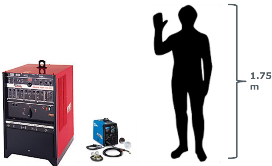
Figure 9. Size comparison of a transformer-based and an inverter-based arc welding equipment, both delivering the same function.
