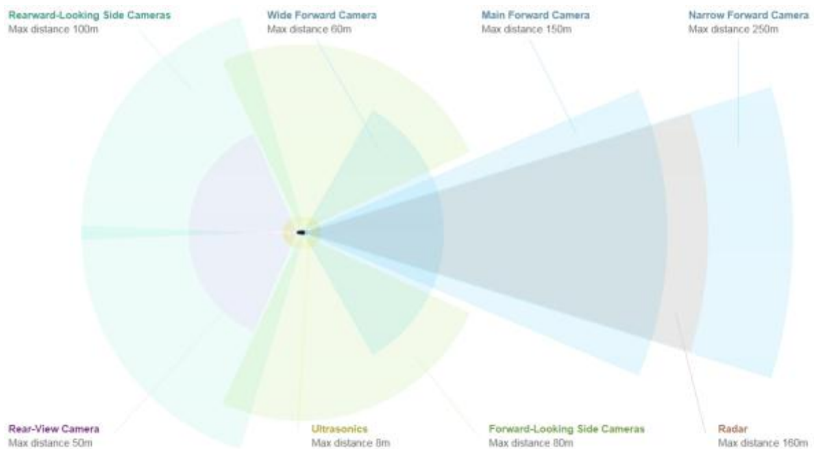
Figure 51 – Cameras and sensors in Tesla’s self-driving car (Credit: Tesla)
