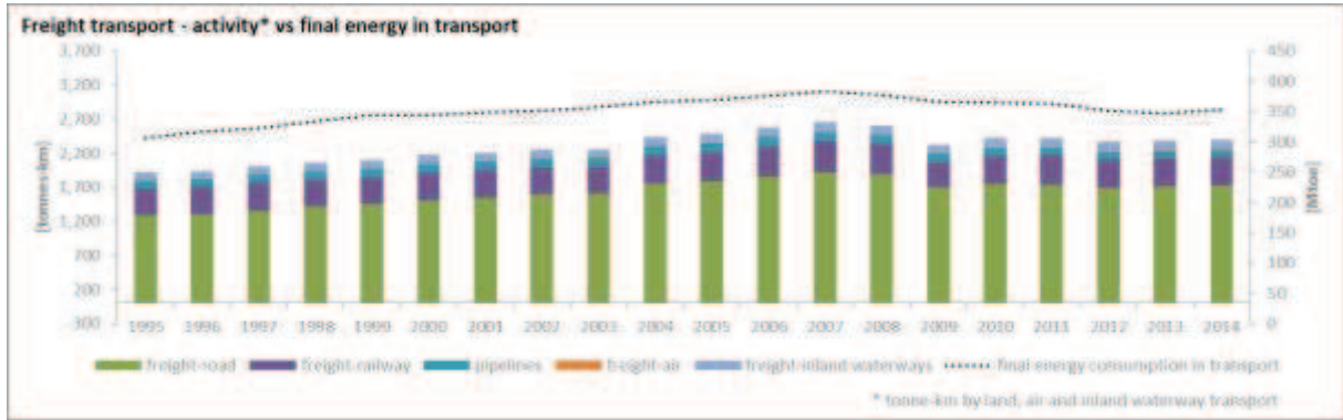
Figure 3.3.14: Evolution of final energy consumption in transport vs. tonnes-km per type of transport in the EU28 (Source of data: Eurostat, DG MOVE Transport in Figures)
