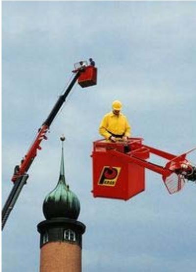
*Work platforms assembled with loader cranes*
